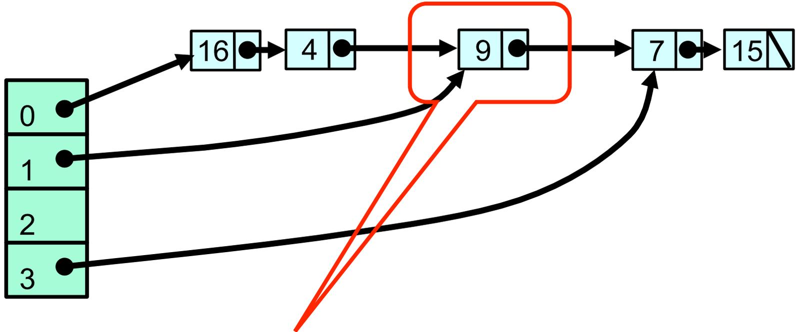
**Problem: how to remove a node pointed by 2 sources using CAS**
